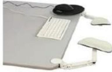
Provides arm support without restricting motion. Includes clamps for work surfaces up to 1-5/8" thick. Provides 17" of reach and 3" of vertical adjustment. Holds up to 35 lbs. \*Tall clamps attach to thick surfaces up to 2-1/2".
