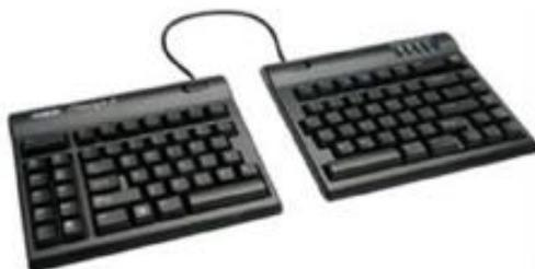
Can be fixed together with pivot tether that allows adjustment of opening angle, but can also adjust to up to 9" after removal of tether. Separate 10-key is available, USB compatible.
